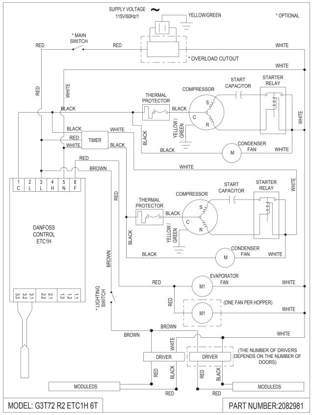
REV.00 Wiring Diagram
