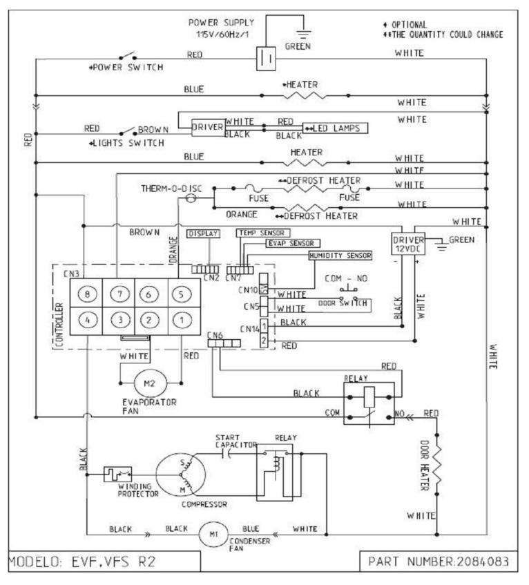
REV.00 Wiring Diagram
