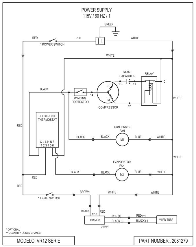
REV.00 Wiring Diagram
